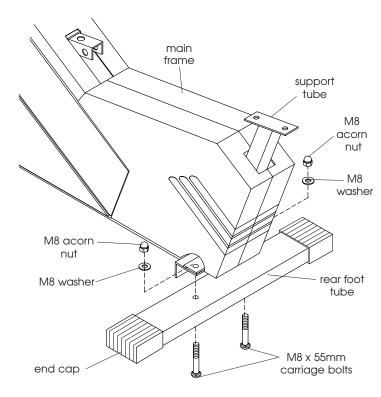
Figure 2 - Install Rear Foot Tube
